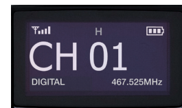
Informative display shows the channel number and the frequency
