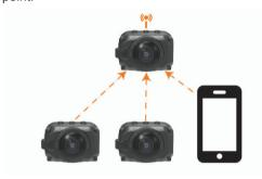
You can also set up a camera network using an existing Wi-Fi network. The app and all cameras connect to the Wi-Fi network. This option is useful when you want to provide internet access to your mobile device while controlling your cameras.
