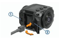
3 Plug the small end of the USB cable into the micro-USB port ② on the camera.
