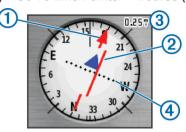
The course pointer ① indicates your relationship to the course line leading to the destination. The course deviation indicator (CDI) ② provides the indication of drift (right or left) from the course. The scale ③ refers to the distance between dots ④ on the course deviation indicator, which tell you how far off course you are.
