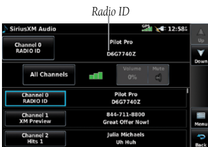
Accessing the SiriusXM Radio ID (Channel 0)
